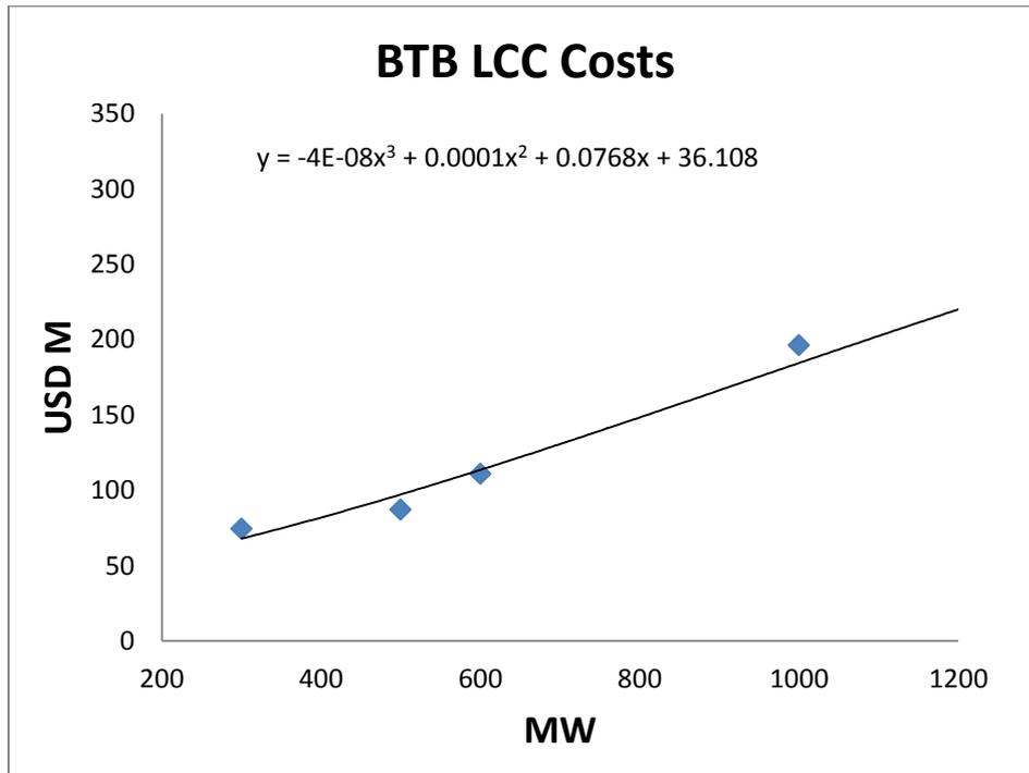
**Figure 7.2: BTB LCC costs as a function of Transfer Capacity (MW)**
