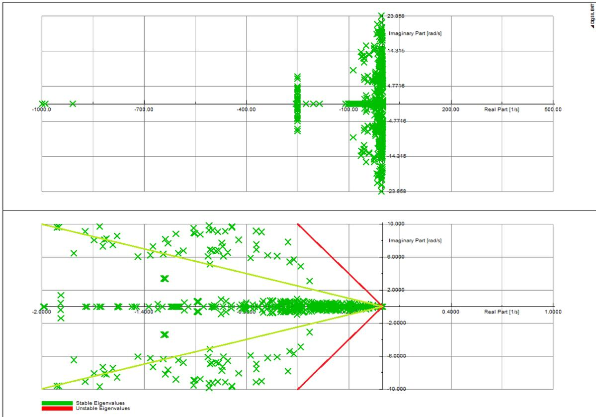
**Figure 4.5: Modal analysis result: eigenvalue plot (the red lines in the bottom figure indicate the target damping of 5% and the green lines indicate the target damping of 20%)**
