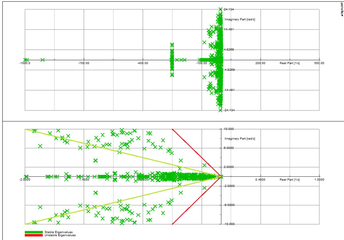
**Figure 4.6: Modal analysis result: eigenvalue plot (the red lines in the bottom figure indicate the target damping of 5% and the green lines indicate the target damping of 20% )**
