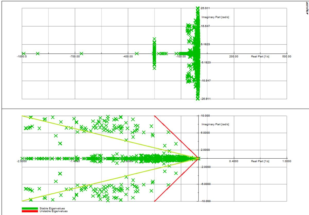
**Figure 4.4: Modal analysis result: eigenvalue plot (the red lines in the bottom figure indicate the target damping of 5% and the green lines indicate the target damping of 20% )**
