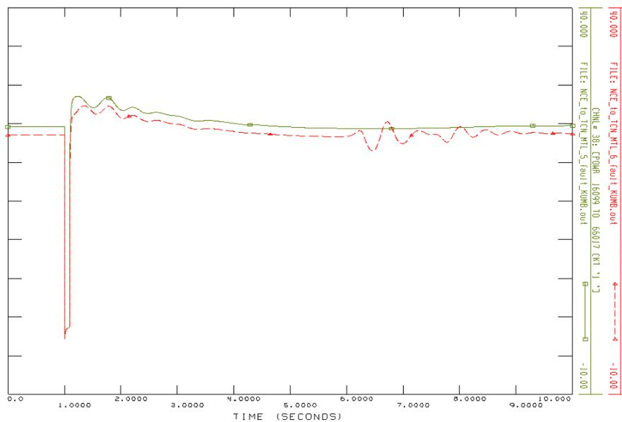
**Figure 4.19: Example of limitation because of transient stability (case “NIGELEC\_NCE to TCN”)**
