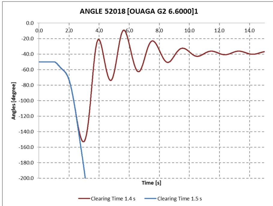
**Figure 4.14: Angles of the critical unit for case #9 (fault at FERKE cleared with tripping of transformer FERKE 225/90, 2016 peak inter-reinf scenario)**
