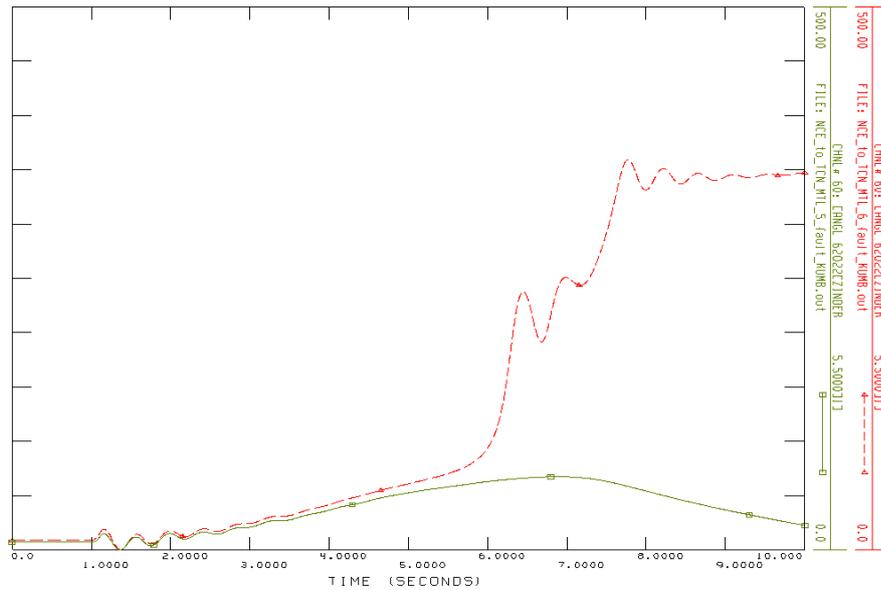
**Figure 4.18: Example of limitation because of transient stability (case “NIGELEC\_NCE to TCN”)**
