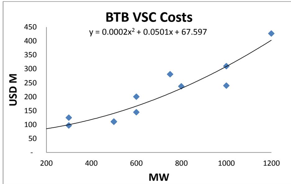
**Figure 7.1: BTB VSC costs as a function of Transfer Capacity (MW)**
