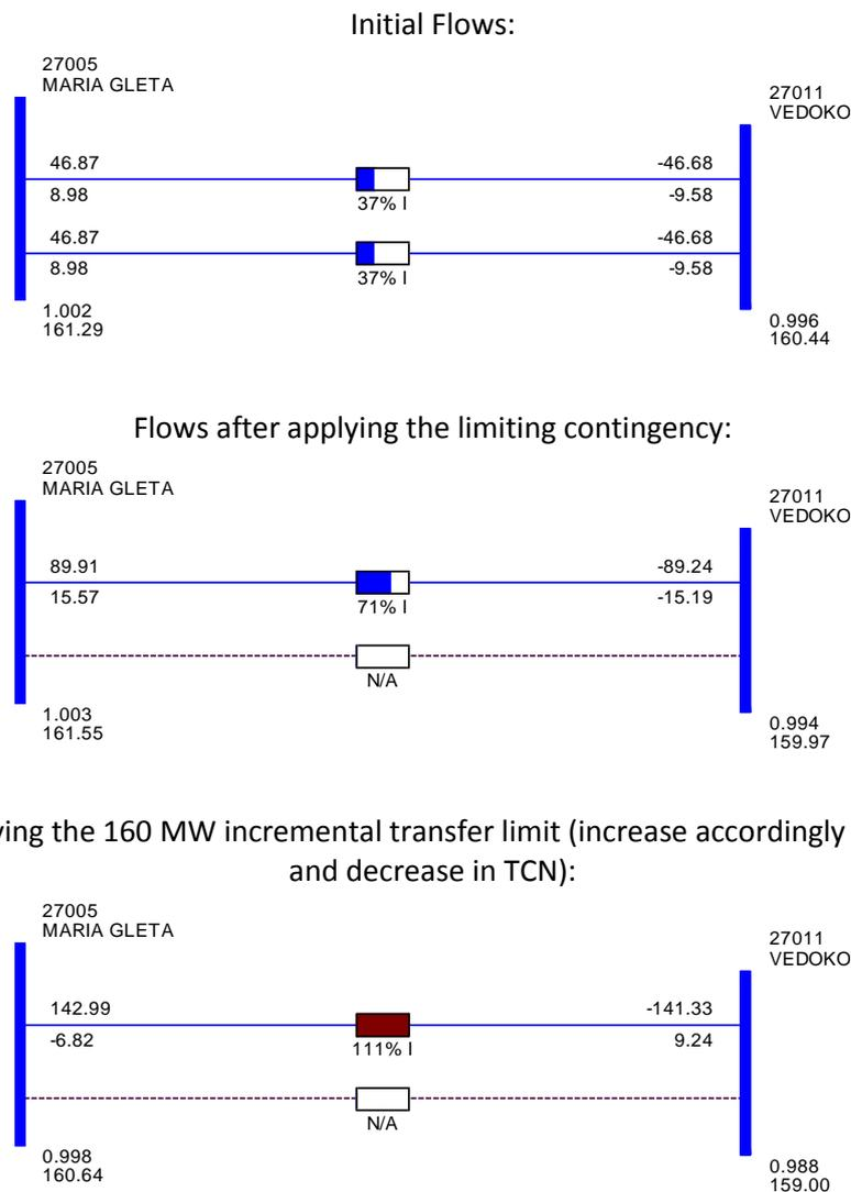
**Figure 4.13: Example of transfer limit calculation (case “CEB to TCN”)**
