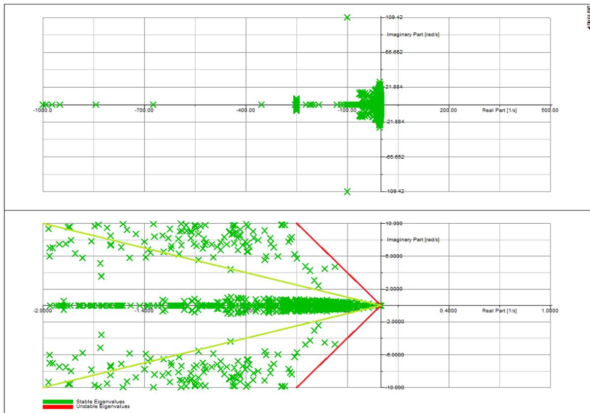
**Figure 4.7: Modal analysis result: eigenvalue plot (the red lines in the bottom figure indicate the target damping of 5% and the green lines indicate the target damping of 20%)**
