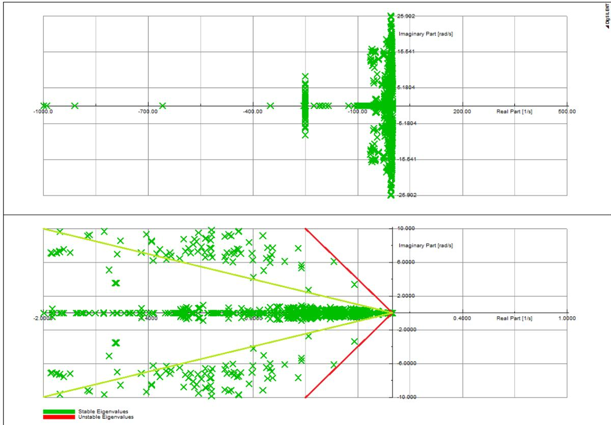
**Figure 4.3: Modal analysis result: eigenvalue plot (the red lines in the bottom figure indicate the target damping of 5% and the green lines indicate the target damping of 20%)**
