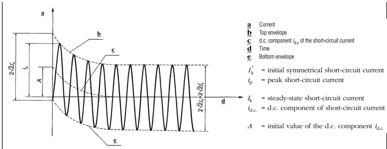
In case of d.c. components higher than 20% they shall be clearly stated in the requirements when specifying the circuit breakers: this requires that suitable breaker tests are performed. According to the IEC standard, the selection of the circuit breaker requirement is made on the basis of the “rated short-circuit breaking current” intended as the R.M.S. value of its A.C. component and specifying the % d.c. component at the instant of contact separation.
