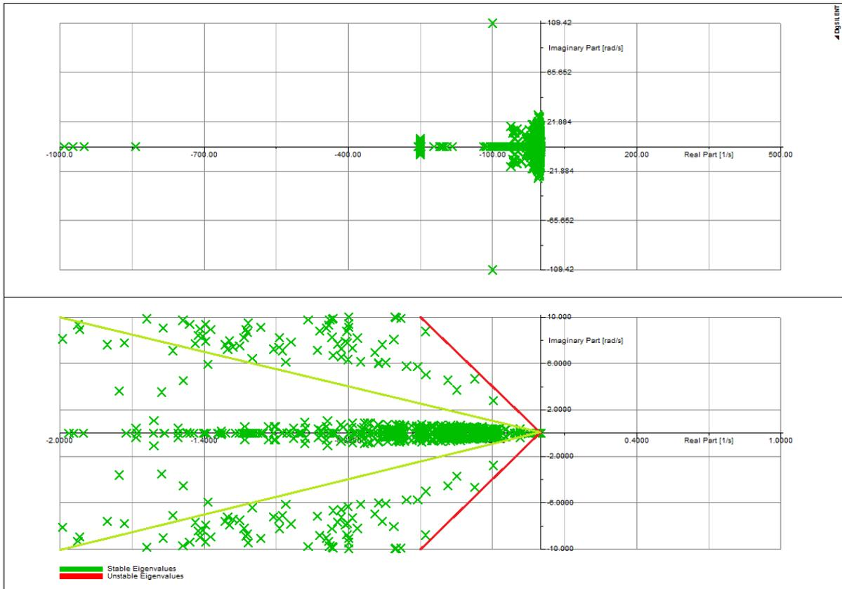
**Figure 4.8: Modal analysis result: eigenvalue plot (the red lines in the bottom figure indicate the target damping of 5% and the green lines indicate the target damping of 20%)**
