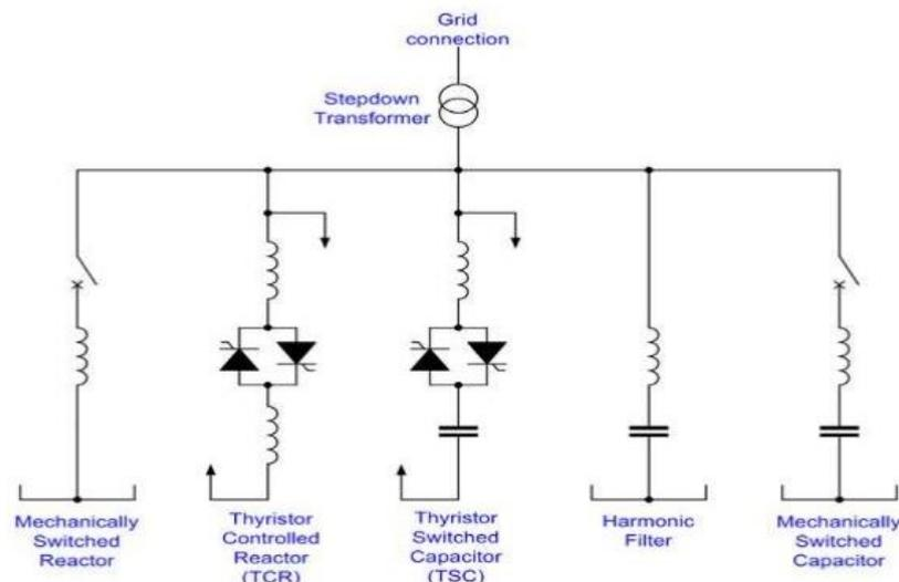
**Figure 7.3: Example of SVC Configuration**
