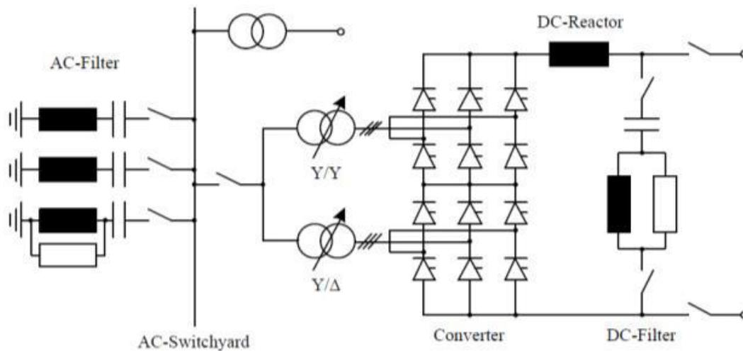
**Figure 6.1: Typical LCC-HVDC configuration with a single 12-pulse converter**
