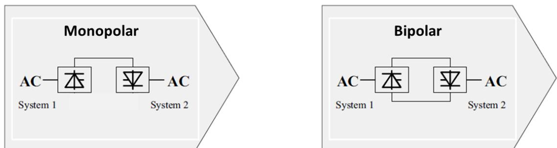
**Figure 6.3: Back-to-back HVDC System Scheme**
