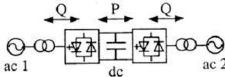
**Figure 6.2: Typical VSC-HVDC configuration**
