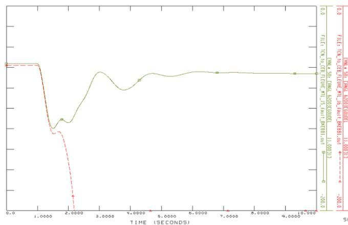
**Figure 4.17: Example of limitation because of transient stability (case “TCN to NIGELEC-FLEUVE”)**
